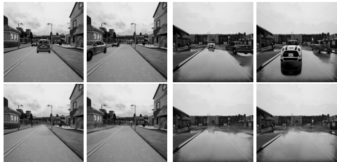
Fig. 1: Images at the same location with different dynamic content such as cars or pedestrians (top row) can be converted into the same static image, i.e. , a dynamic-object-invariant space (bottom row).
